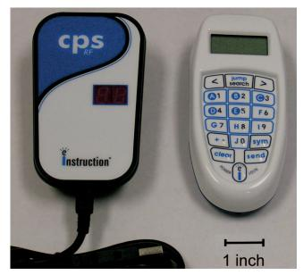
Figure 1. CPS receiver (left) and keypad.
