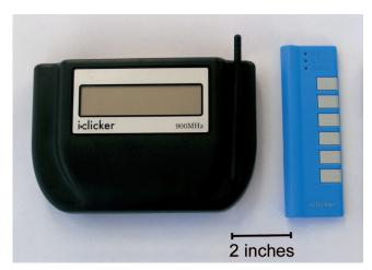
Figure 5. iClicker receiver (left) and keypad (right).
