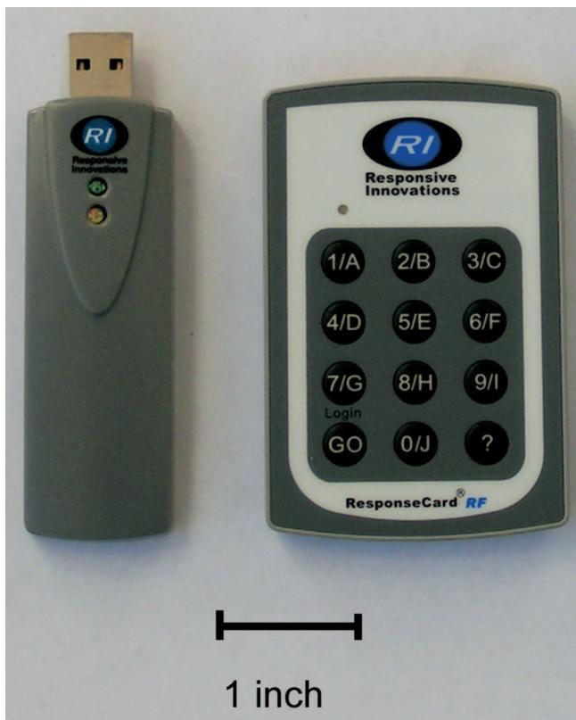
Figure 3. TurningPoint receiver (left) and keypad (right).
