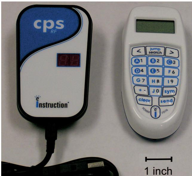
Figure 1. CPS receiver (left) and keypad.
